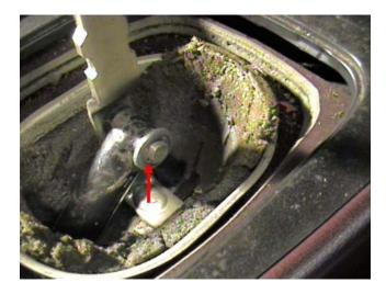
b. On 968s, remove the spring clip (17) from the groove on the shift lever pin. Remove the washer (18) and bushing (19) from the shifter rod. You may have to slide the shifter rod off of the shift lever pin to remove the bushing. Remove the other bushing from the shifter rod and the remaining washers from shift lever pin.
