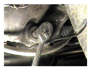
11. When you get the strainer out, inspect the strainer for debris built up on the outside of the screen. You can see from the picture below that this particular strainer is very clean. You may find some debris at the base of the strainer (second picture below) which may be cleaned out using a small probe. However, be careful not to poke a hole in the strainer while you're cleaning that area.
