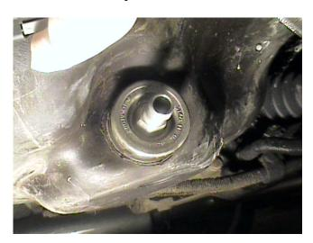
10. Using a 17 mm deep socket and ratchet or 17 mm wrench on the hex of the nozzle, turn counter-clockwise to remove the nozzle and strainer assembly. Make sure you have a container underneath the tank. The bottom of the strainer assembly is below the level of the nozzle so, some additional fuel (a small amount) will drain from the tank when the strainer is removed.
