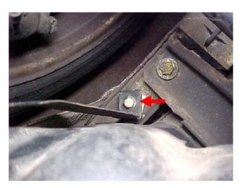
5. Locate the fuel line going from the bottom of the fuel tank to the suction of the fuel pump and pinch the rubber fuel line using a hose clamp (as shown below).
