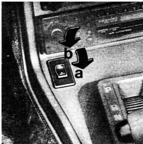
2. On late model 944s with the larger switch, disconnect the sunroof switch plug as follows:
