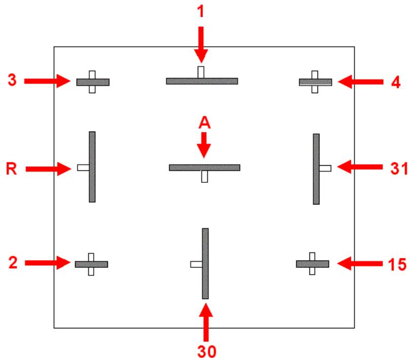
5. If the correct supply voltages are present and the correct output voltages are not present, the main sunroof relay is most likely faulty and needs to be replaced.
