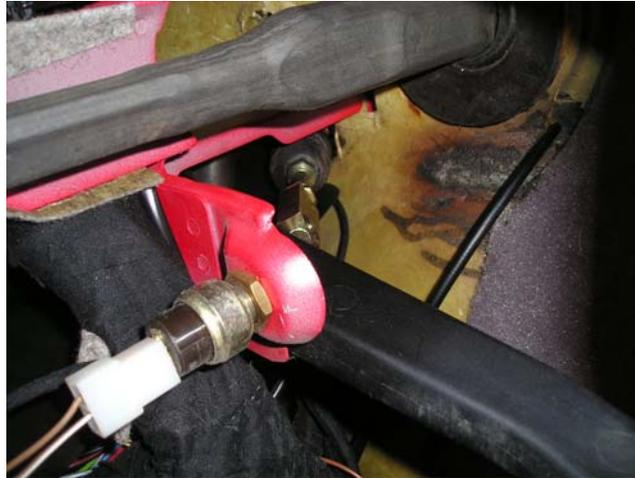
Tighten the nuts with the concave washers behind them. I used a universal joint on the socket wrench, but I found a ¼ inch drive socket worked without the universal attachment. Your mileage may vary.
