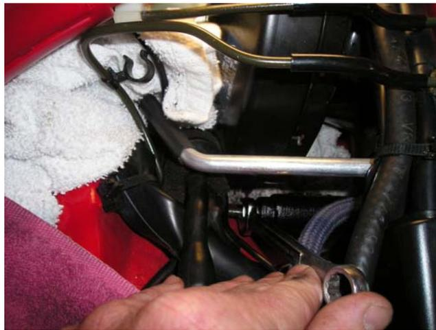
10. Using a universal joint type adapter on your socket wrench, remove the two 13mm bolts holding the clutch master cylinder to the firewall. Place a magnet near the socket as you work in order to catch the nut and concave washer. I stuffed rags in the open spaces below the master cylinder to help catch flying parts.
