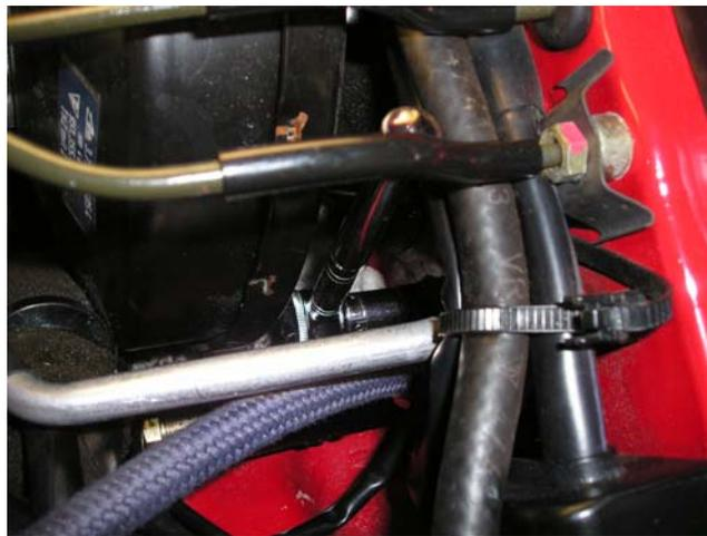
7. Install hard line to front of clutch master cylinder with 12mm-flare nut wrench. Have patience, as there is little room to work here.
