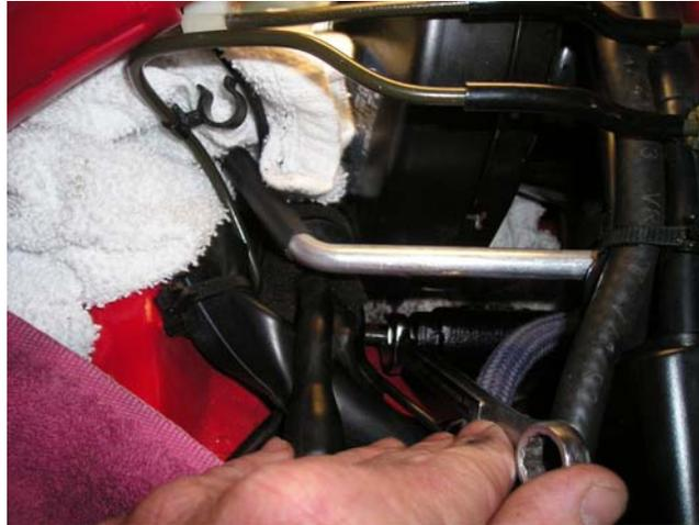
8. Install blue hose to brake fluid reservoir. Be careful not to over-tighten and break the plastic nipple.
