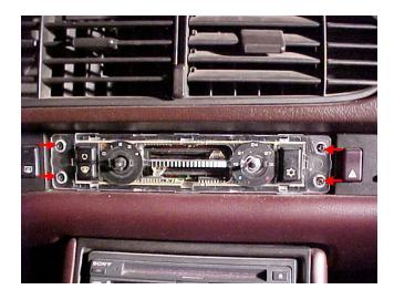
4. You'll find an electrical connector plug on the back of the temperature control unit. Disconnect the plug and the TCU should slide right out of the dash.
