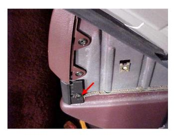
4. Carefully remove the rectangular trim cover next to the passenger side vent control lever using a small flat tip screwdriver.
