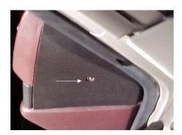
3. Behind the side trim panel, you will find three (3) Phillips head screws. Remove the bottom screw which holds the trim panel in place.
