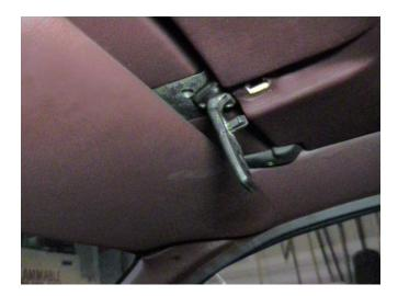
3. From inside the car, push up on the back of the sunroof and slide it off of the wind deflector and front guides.
